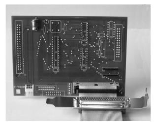
Below is the PCI-7200 card on the left, the Daughter Board on the right and the spacer/screw assembly. Note the matching holes in the Daughter Board and the PCI-7200 card. The small washer is included for a precise fit and must be installed between the boards, at one end of the spacer or the other. This may already have been done prior to shipping.
