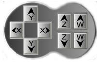
These buttons are what allow you to initiate a manual transit or jog movement from the console of the computer that runs the machine. In transit mode, holding the button down will continuously move the machine. In jog mode, each time a button is pressed the machine will move according to the jog incre-
