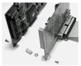
Insert the Daughter Board on to the 40-pin connector of the PCI-
