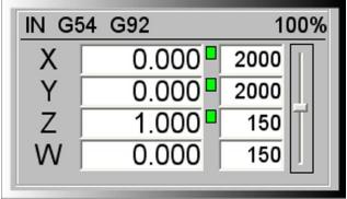
Alternately LZ may be set by shifting MZ the desired amount using G92.1. Using G92.1 it is not necessary to move to the workpiece first.
