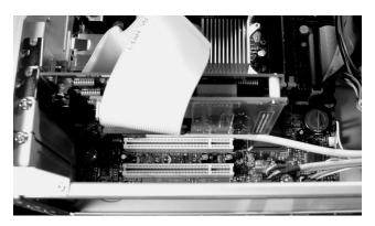
**Very Important!** Install the 37 pin cable from the control box into the daughter card (BLUE) connector, not the PCI (BLACK) connector. The cards have different power and ground pins and the cards will be damaged if connected incorrectly.
